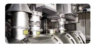
3.0 m ploughshare mixer with screw type dosing; exhaust gas filtering with a large cleaning flap
