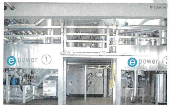
Cryogenic grinding plant; cold grinding of plastics and other elastic materials as well as temperature-sensitive
