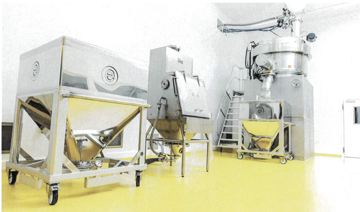
Ebbecke cleanroom concept, showing a pharmaceutical mixer (known as an API mixer).
